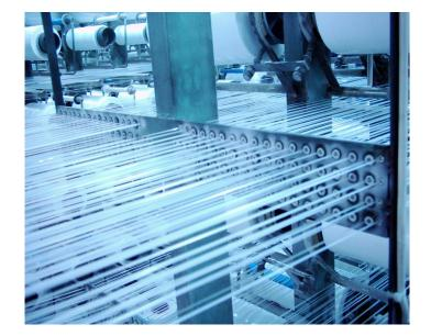
1500 horizontal spinning coil adapter and tension mechanism, big bag for warping creels.
