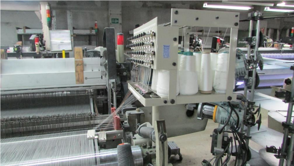
20 bobbins Leno Creels installation. [Picanol Optimax]
